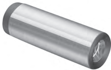
Flat Vent (Ground Flat Helps to Relieve Trapped Air)
