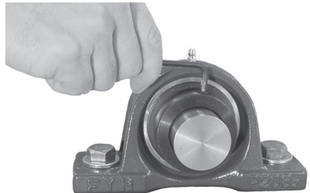
Fig. 14.10 Installing eccentric locking collar
